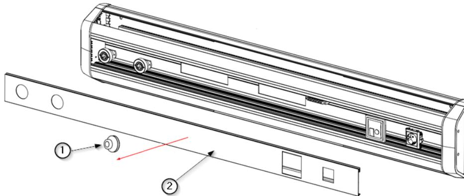
Fig.3 Removing the central cover of the gas rail
