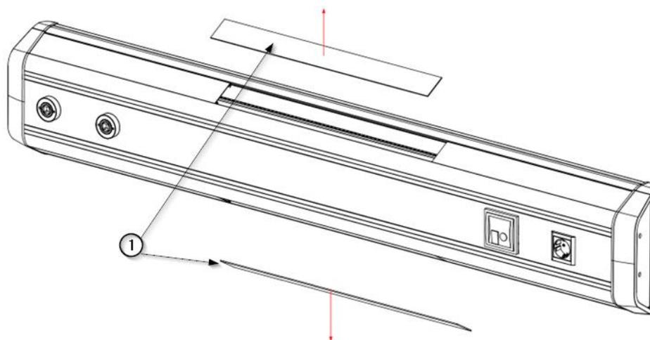
Fig.1 Removal of upper and lower diffusers
