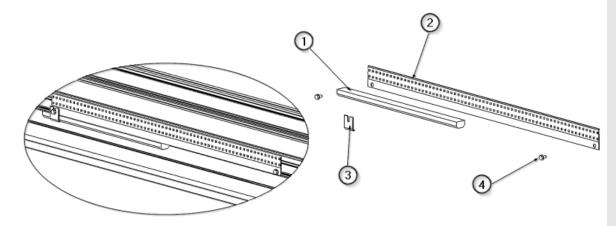
Fig.4 Replacing LED strips and controllers
