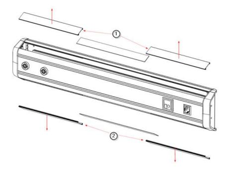
Fig.2 Removal of top and bottom coverings
