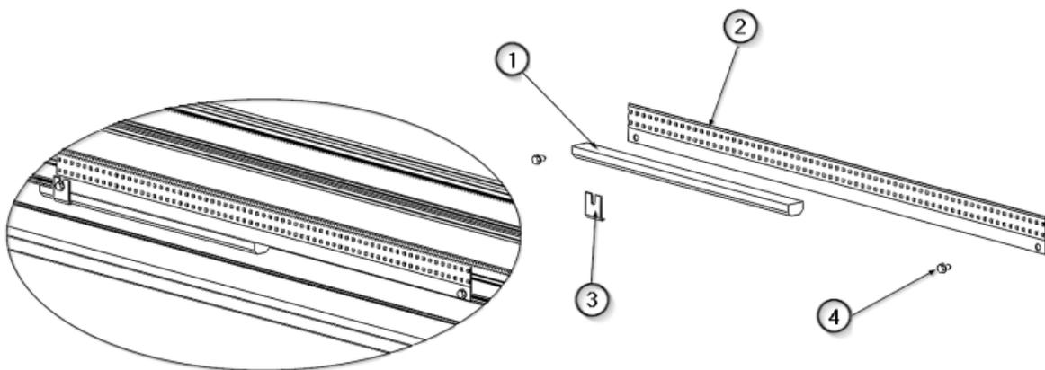
Fig.4 Replacing LED strips and controllers
