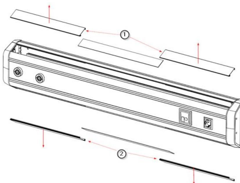
Fig.2 Removal of top and bottom coverings
