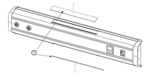
Fig.1 Removal of upper and lower diffusers
